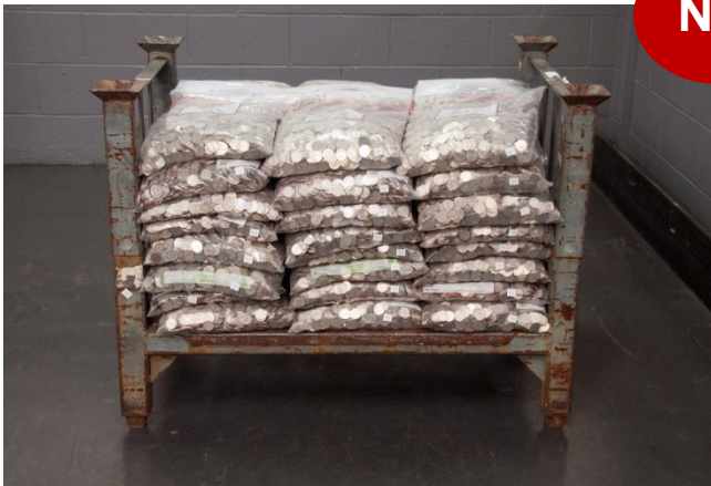
INCORRECT —The plastic bags are stacked on the pallet with all labels facing inward.
